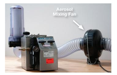
NOTE: Use the variable transformer to control the flow output of the aerosol-mixing fan to  $\leq$  10 CFM.
