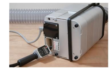
6. Place the photometer probe into the rack interface of the supply blower as shown below:
