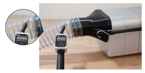
5. Record the challenge concentration used and adjust the photometer to read the upstream concentration as 100%.
